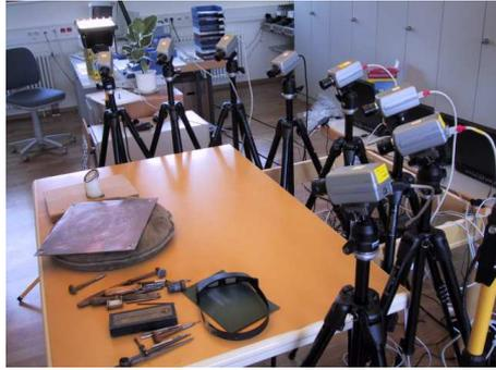
Figure 6: A camera setup for the recording of a copper engraving craftsman.
