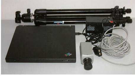
Figure 3: *The module-components of our system. Tripod, laptop, camera, battery and inter-module cabling. The total weight is less than 10 kg. It all fits into a backpack for easy transportation.*
